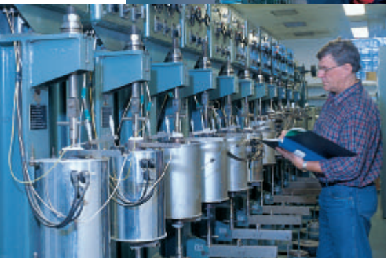
1. Furnace for diamond coating of cemented-carbide inserts at Sandvik Coromant in Västberga, Stockholm.
